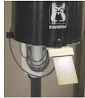
The leaf wetness sensor is designed to be mounted on the North side of the weather station. The bracket provided with the sensor insures a solid and secure installation.
