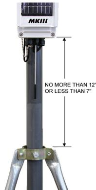
3. Rotate the assembly until the solar panel faces TRUE SOUTH, TRUE NORTH if you are in the southern hemisphere. Secure the support tube to the assembly to prevent it from rotating.
