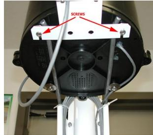
2. Mount the support tube as indicated; A tripod is shown. You can also use U-bolts or a Mono Mount. Insert the neck down end into the sensor assembly until it bottoms with the retaining screw in the slot. Tighten the screw.
